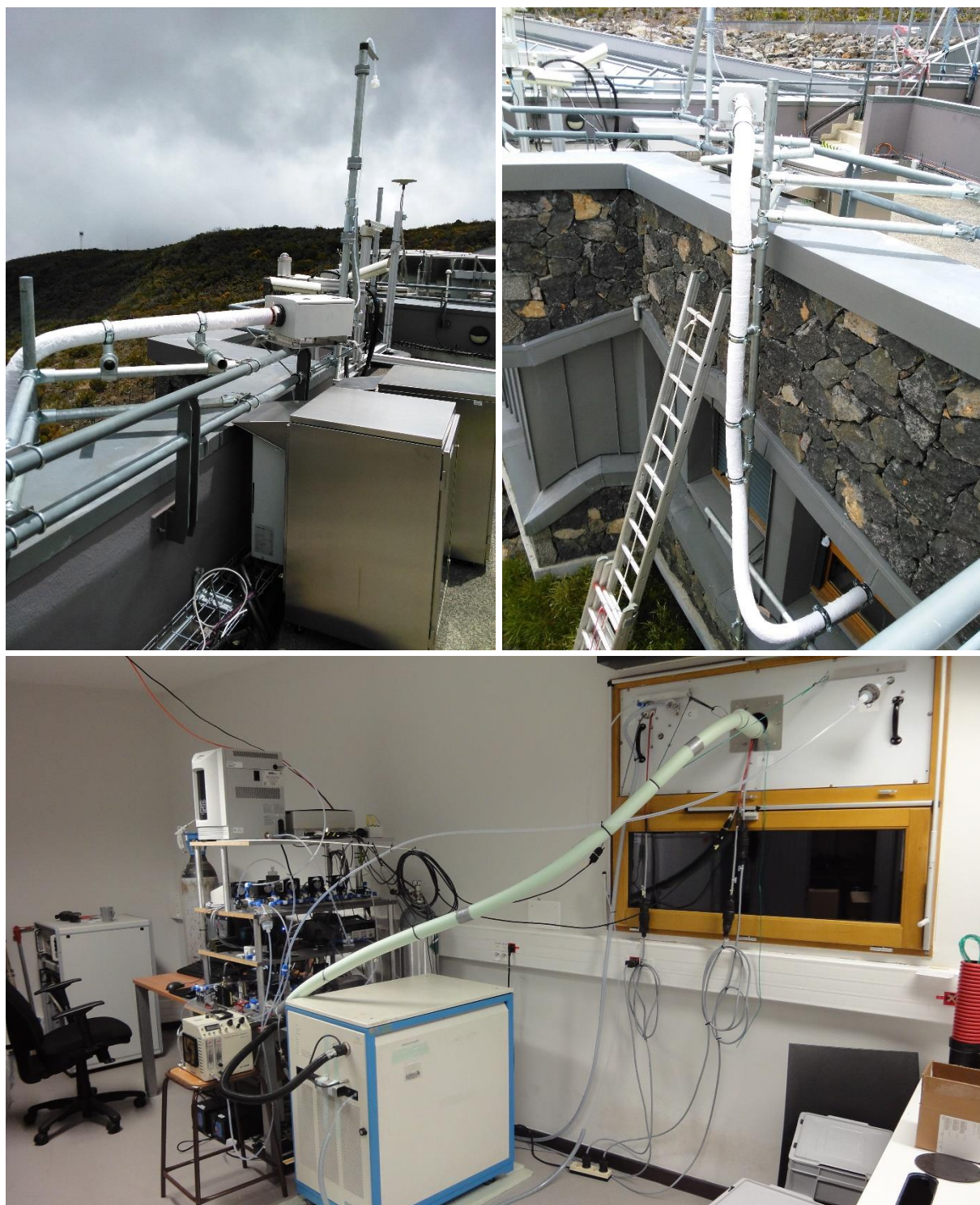
Figure 2. Top left: air sampling from the roof of the observatory; Top right: support structure to guide the sampling line; Bottom: (O)VOC measurement set-up in the laboratory (hs-PTR-MS and associated set-up for zero and calibration measurements and remote instrument control).
