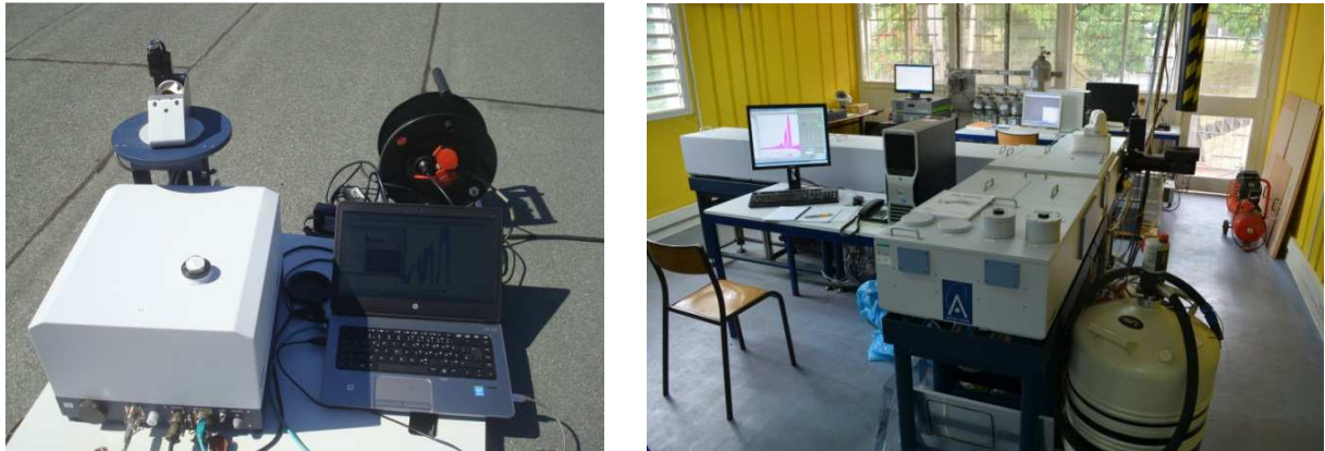
Figure 1: EM27/SUN spectrometer (left) and Bruker IFS 125HR spectrometer (right), both performing side-by-side measurements.
